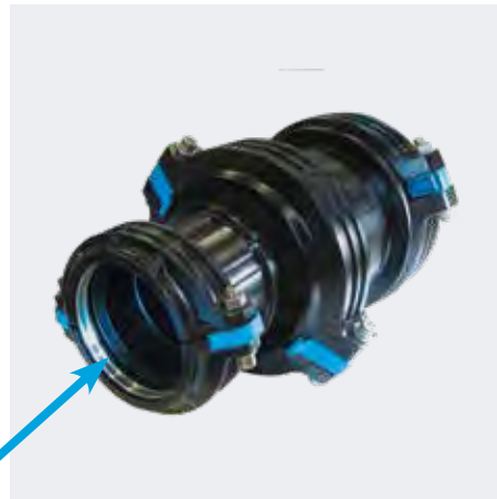
Insert the Reducer in the desired position, reassemble the clamp halves and tighten the bolts and nuts at a torque value of 11 lb-ft.
