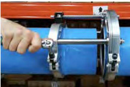
Step 4: Tighten both sides of the UnipipeEZ Install Tool with socket wrench.
