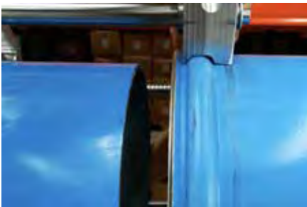
Step 2: Align groove on socket pipe to groove on UnipipeEZ Install Tool.
