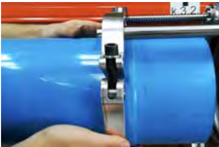
Step 3: Fasten both sides of the UnipipeEZ Install Tool around the pipe.
